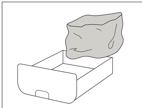
Pull out the waste litter drawer and line it with a litter liner bag. **Push the liner all the way down** and fit it firmly on the sides to prevent blocking the internal sensors. Place the charcoal air filter pouch in the drawer's middle compartment.
