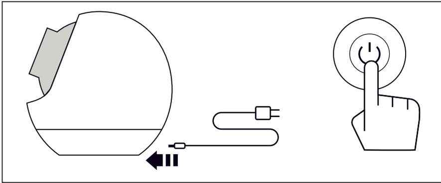
Plug in the power adapter, then **long press the POWER button for 3 seconds** to turn on the machine. Make sure to **place the machine on a solid flat surface** for the scale and safety sensors to work properly.
