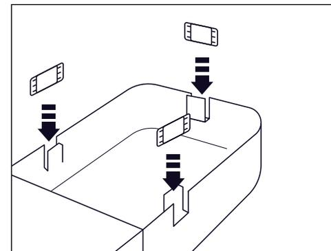
Push clips firmly down into their slots to secure the liner bag and **ensure they are not sticking up**. Gently push the waste litter drawer back into position.
